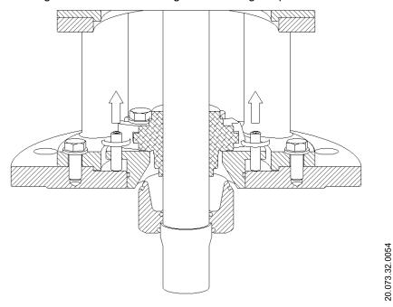
18. Tighten the mechanical seal set screws and remove the plastic strip or metal tabs. The agitator is now ready to operate.
