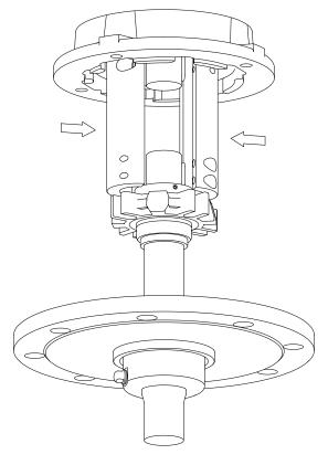
Place the Allen bolts in the coupling and tighten carefully in a cross pattern maintaining the coupling faces parallel to each other. Separation between the faces when tightened should be around 2mm.
