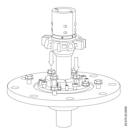
10. Once the bottom shaft is properly fixed, the shaft coupling can be removed. First remove the Allen keys and use a flat screwdriver or similar tool to pry open both halves of the coupling.
