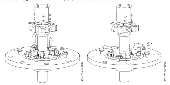
15. Install the new mechanical seal in place, preferably with the plastic strip insertion point oriented upwards for ease of access.
