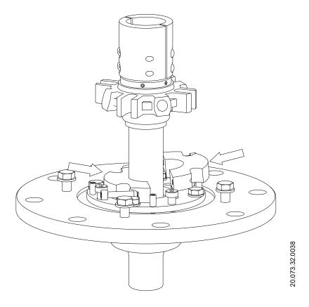
9. Screw the fixing bolts in and slightly tighten them so that the fixing tool is flat against the flange. Then, tighten the Allen screws and after that, tighten the hexagonal screws to completely fix the tool to the flange. This will fix the shaft to the agitator flange so the coupling can be removed so it is important to follow the instructions correctly.
